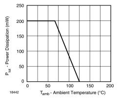
Figure 1. Admissible Power Dissipation vs. Ambient Temperature
